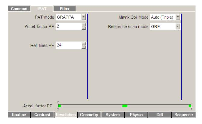
**Reference scan mode:** If iPAT is enabled, the reference scan acquisition scheme can be selected here. "Single-shot" EPI (Siemens default for accel. factor 2) is the fastest but limits the number of reference lines. "Segmented" EPI (Siemens default for accel. factor >2) allows for more reference lines, but increases motion sensitivity. "GRE" offers high SNR and is insensitive to motion, but may result in other artifacts (this option is currently experimental).
