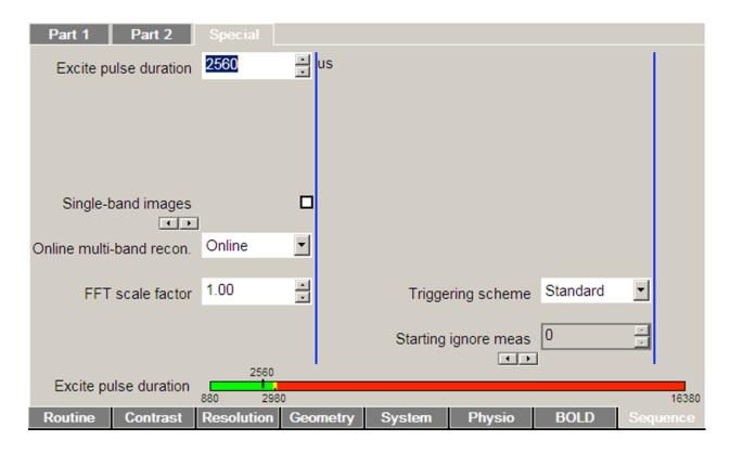
**Excite pulse duration:** The required RF pulse voltage increases linearly with the multi-band acceleration factor. Here the pulse length of the excitation RF pulse can be manipulated manually at the cost of  $T_E$  and bandwidth.
