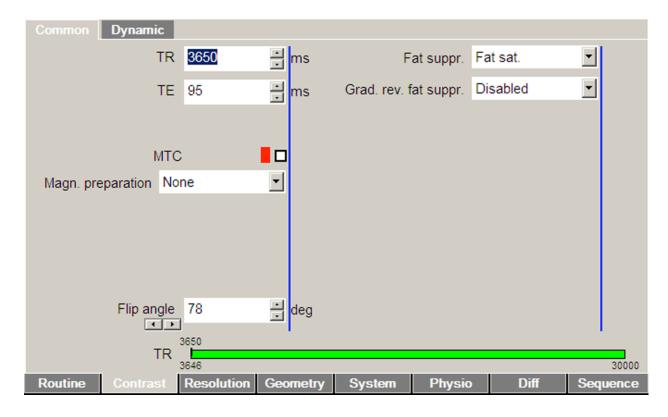
**Grad rev. fat suppr. (SE/diffusion only):** If enabled, the polarity of the slice select gradients will be reversed between excitation and refocusing. This can provide effective fat suppression at no cost in time or SAR. It can also result in signal losses in areas of B0 inhomogeneity. Typically it is most useful at 3T.
