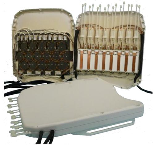
**Figure 13.** Half of a local, 32 channel receive array is shown next to half of a local, 16 channel transmit array (above). The packaged assembly is shown below.
