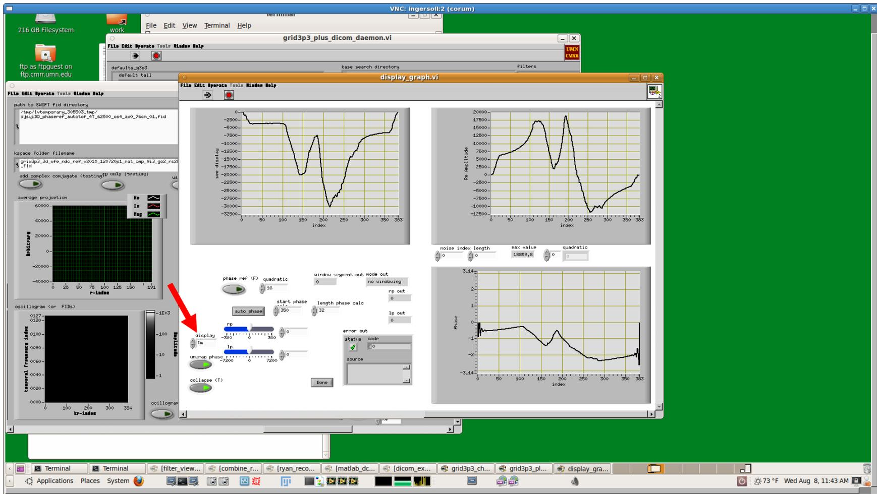
The window `display_graph.vi` will open. The upper left shows imaginary (by default), the upper right shows the real, and the lower right shows the phase of the average projection.
